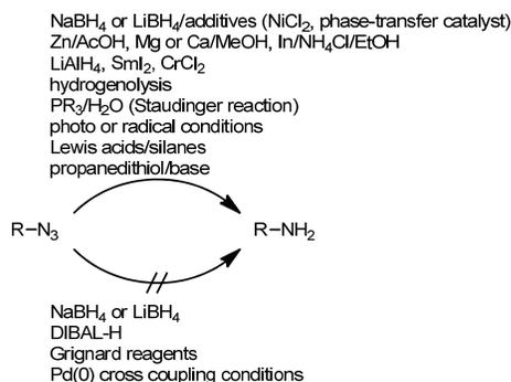
**Scheme 35:** Typical procedures of azide reduction to amine, and the conditions azides are tolerant.
