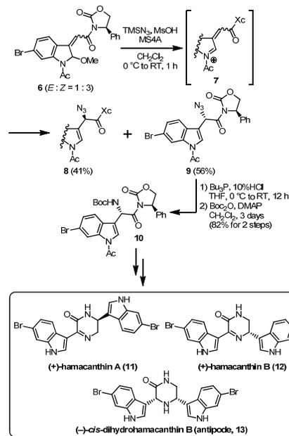
Scheme 6: 1,4-Azidation of eniminium intermediate in total syntheses of marine bisindole alkaloids by Kawasaki et al.
