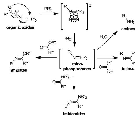
**Scheme 30:** Typical reaction mechanisms of Staudinger reaction and the following aza-Wittig reaction.
