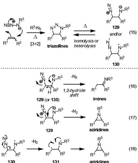
**Scheme 24:** Reaction mechanisms of azide-olefin [3+2] cycloaddition and further transformations.
