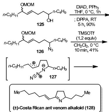
**Scheme 23:** Total synthesis of Costa Rican ant venom using allyl cation-mediated Schmidt-type reaction to directly form unsaturated imine by Tanimoto et al.
