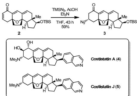
Scheme 5: 1,4-Azidation in a model study of total syntheses of costistatins A and J by Yamashita and Hiramata et al.
