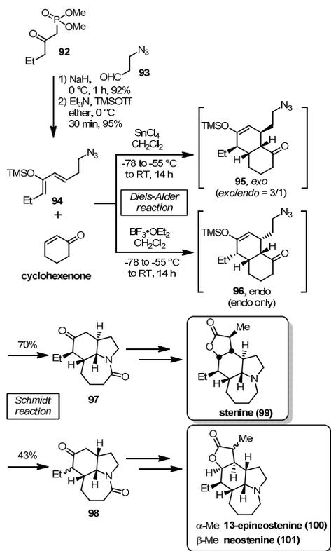
Scheme 19: Total syntheses of stenimona alkaloids by way of Diels-Alder reaction–intramolecular Schmidt reaction cascade by Aubé et al.
