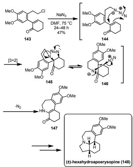
**Scheme 26:** Total synthesis of hexahydroapoerysopine through azide-olefin [3+2] cycloaddition followed by ring-expansion reaction by Tu et al.
